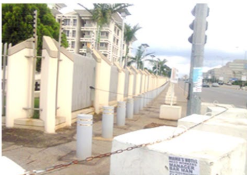
Plate VI: The fence creates a territorial identity thereby establishing ownership and control of the space within the fence. Engineered blocks and bollards are used as vehicle barrier. These increase deterrence (Ministry of Foreign Affairs, Abuja). Photo credit: Samuel Ebong
