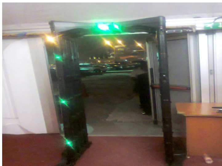
Plate VIII: M-scope metal detector for access control during a function (This Day Dome, Abuja. Photo credit: Samuel Ebong)
