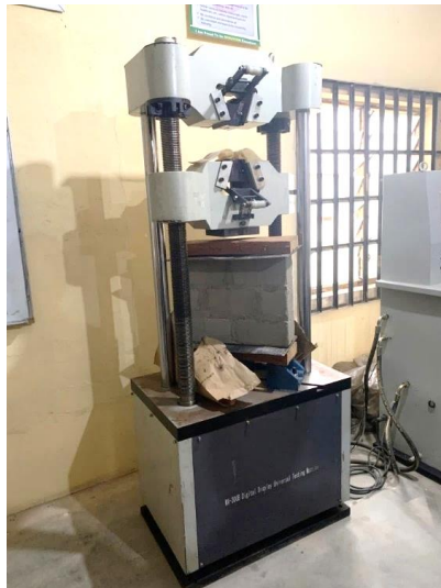
Figure 4: Test setup adopted for uniaxial compressive strength test of concrete block prisms.
