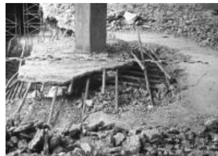
Figure 1b: Punching and post punching shear mechanisms (Source: Mirzaei and Muttoni, 2008)
