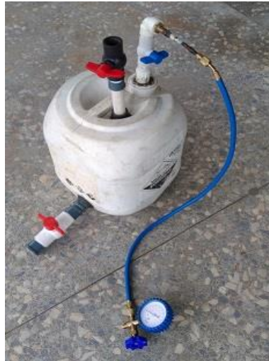
Figure 9.2: The developed anaerobic digester
